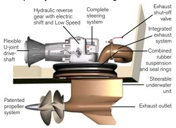
The Volvo Penta IPS has been developed and is manufactured as a complete integrated system from the helm to the propeller cone – engine, propulsion unit incl. gear box, propellers, exhaust and seawater system, steering, instruments and controls. Installing the units is easy. Our own tests show installation time reduced by well over 50%.
