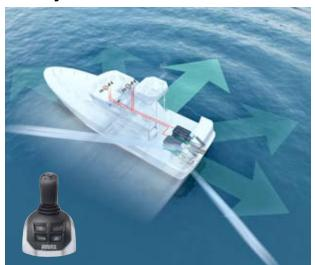
With the joystick the helmsman can now maneuver the vessel in any direction at low speed – with just one hand. The joystick is coupled to a sophisticated and specially developed software that individually commands the electronically engines and the pod units to steer, throttle and shift gears independently, making the boat move in any direction the driver wants – sideways, diagonally, forward, backward or rotate.
